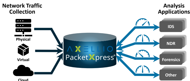
Figure 2: PacketXpress — High-speed network packet data capture, storage, distribution, control, and analysis solution
