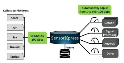
Unlike today's top-end wideband recorders, SensorXpress can stream data simultaneously on disk and off disk at over 100 Gbps, allowing for a consumption of a larger volume of RF data from multiple sensors. SensorXpress also stores data at a much higher density without quality loss. Being sensor, analysis tool, and spectrum agnostic allows you to extend the useful life of your existing collections and analysis infrastructure while maximizing its capabilities.
