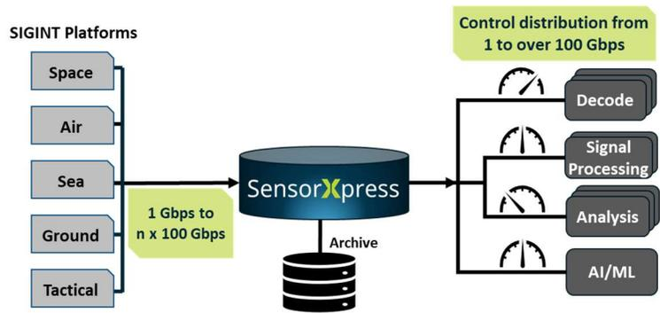
Unlike today’s top-end wideband recorders, SensorXpress can stream data simultaneously on disk and off disk at over 100 Gbps, allowing for a consumption of a larger volume of SIGINT data from multiple sensors. SensorXpress also stores data at a much higher density without quality loss – close to Petabyte in just a 2U form factor. Being sensor, analysis tool, and spectrum agnostic allows you to extend the useful life of your existing SIGINT/ELINT infrastructure while maximizing its capabilities.
